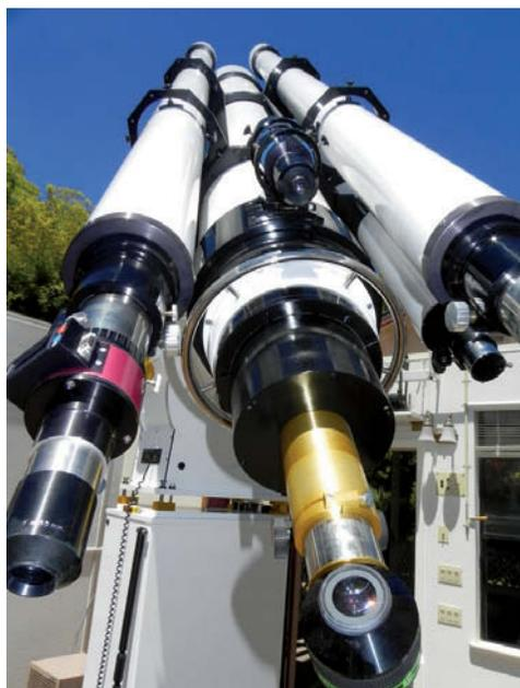
The business end of the 12-inch refractor includes a very large stainless-steel "yacht steering wheel" made by Ed Byers. It allows the observer a convenient handhold for swinging the big telescope and its auxiliary instruments around the sky.
